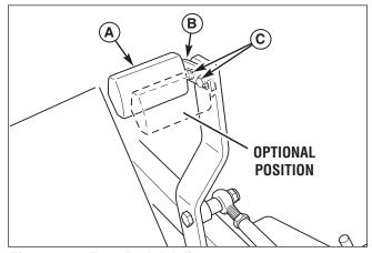
Figure 36. Foot Pedal Adjustment
